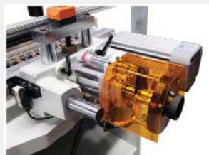
Rotary turret system for quick depth setting
