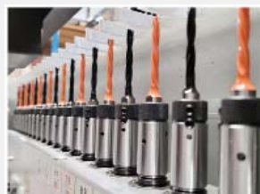
21 spindles with quick change chucks for fast boring pattern changeover
