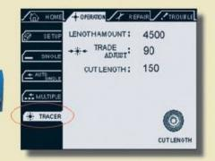
This section It can also to set one desire d cutting size between the defect parts automatically
