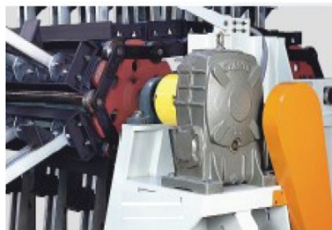
Heavy-duty worm gear reducer to ensure the transmission quality of the machinery, and even in the state of unbalanced load rotation the caterpillar chain for rotation feeding is stable.
