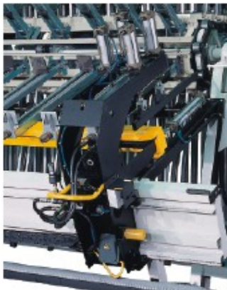
Hydraulic type with top press cylinders.
