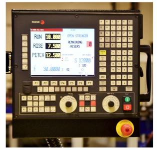
The CSR-750CNC is equipped with a 3-axis Industrial CNC package build by FAGOR AUTOMATION. To make operation of this machine as easy as possible, the CNC unit is preprogrammed for most stair routing applications. However, the CSR-750CNC still retains full capability of editing existing programs and entering new ones.
