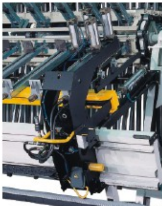
Hydraulic type with top press cylinders.
