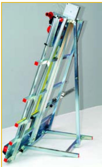
An optional folding stand allows these machines to be moved all over your shop
