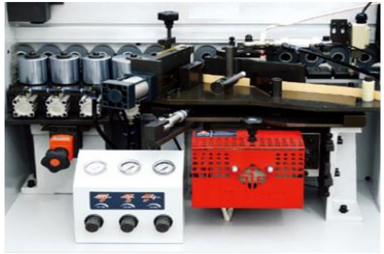
Hot Glue Tank Unit
