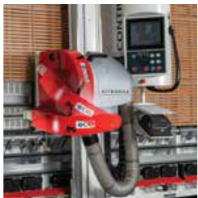
Automatic saw head pivoting is just one feature that automates the sawing process.
