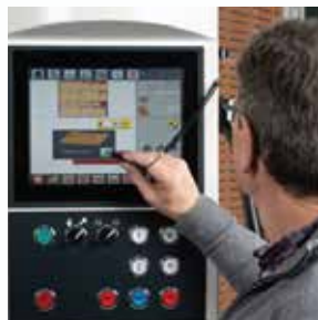
The 12" color touch screen with advanced user interface controls most saw functions.
