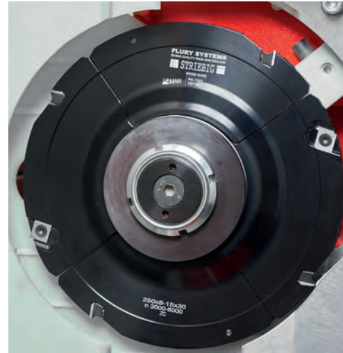
Reversible carbide tips for adjustable grooving tools
