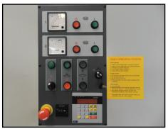
CONTROL PANEL WITH DIGITAL THICKNESS ADJUSTMENT
