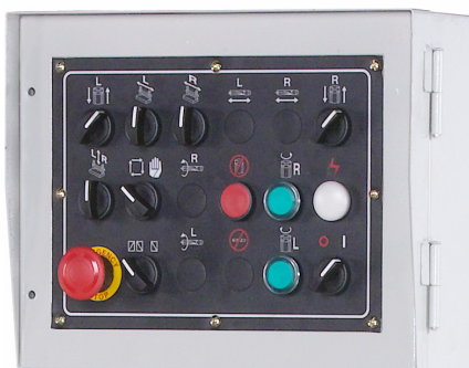
Two set of controller for use Single Table by itself or Both Table at same time
