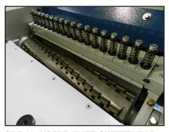
SPIRAL INSERT KNIFE CUTTERHEAD Comes equipped with top and bottom insert knife cutterheads with standard 30x12x2.5mm 2-sided reversible knives. Provides optimum finish with minimal noise
