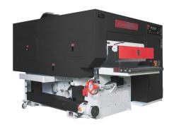
**OPTIONAL CE GUARD**Optional fully enclosed guard cover with limit switches on doors to CE standard.
