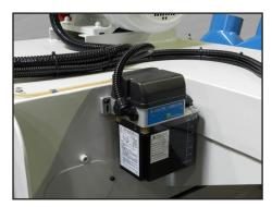
**AUTOMATIC LUBRICATION**Conveyor system is constantly lubricated by an electronic oiler ensuring maximum life with minimum wear
