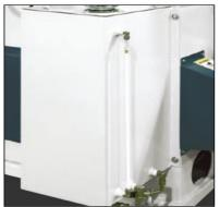
Automatic lubricator provides lubrication and cooling for the sawblade. It also reduces considerable noise level.
