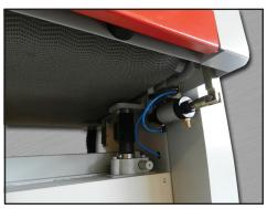
**CONVEYOR BELT TRACKING & HEIGHT ADJUSTMENT SCREWS** Pneumatic conveyor belt tracking to ensure belt does not run off to one side. (4) precision jack screws for table height adjustment.
