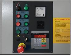
**CONTROL PANEL WITH DIGITAL THICKNESS ADJUSTMENT** - Centrally located control panel for convenient operator access. Includes digital motorized thickness adjustment to 3-decimal places in Inch & 2-decimals in MM. Also emergency stop button, ammeter for load monitoring, and hour meter to aid in maintenance.
