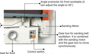
Lifting adjustment handwheel for front worktable. It is easy to elevate the worktable and handwheel which is driven by worm gear
