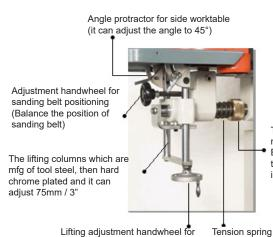
The sand belt can be replaced by the nut quickly. Excellence: it can adjust the tension of sand belt, and increase the stability
