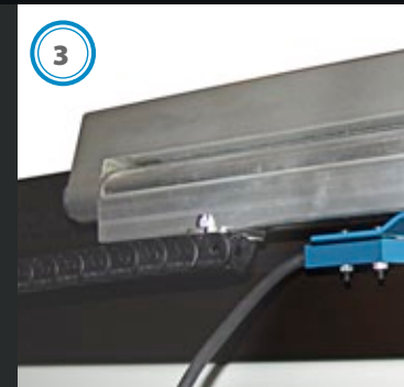
Precision measurement by magnetic tape.
