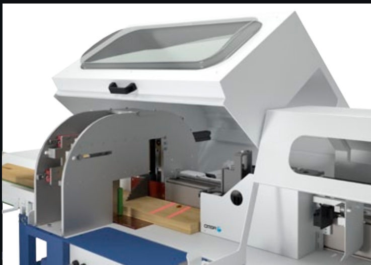
Defecting with trim cut on the two sides.
