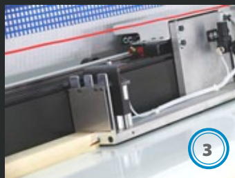
Vertical pneumatic gripper
