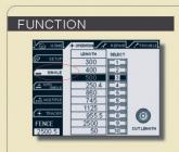
This section is acted as stopper for single size cutting. Just key in the desired size for the cutting length or choice the size from the 10 sets of memory.
