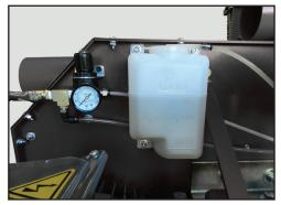
**Blade Spray Mist Cooling System** Is driven by motor, providing fast and convenient adjustment for thickness of cut.
