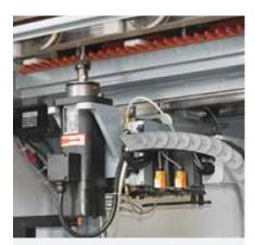
High Frequency Spindle Motor
