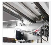
Ball Screw & Linear Guideway Driven by a high speed servo motor in combination with the use of ball serew
