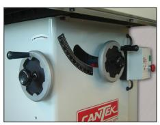
**BLADE ADJUSTMENT HANDWHEELS**
