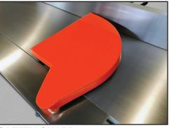
SAFETY GUARD The spring loaded safety guard moves only when the workpiece is being fed. The guard will return to its original position upon completion of the cut ensuring a safe operation.
