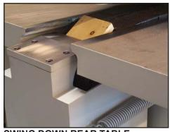
SWING DOWN REAR TABLE Avoids possible damage to the machine by preventing short work pieces from accidentally falling between the table and the chain.
