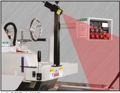
LASER LINE Provides for quick and convenient positioning of cut which also reduces material waste
