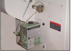
**MECHANICAL CHAIN LUBRICATION** Lubricant flow rate can be adjusted automatically with the caterpillar chain feed speed variation. When lubrication runs out the chain stops automatically preventing damage to the machine.
