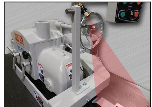
Optional Alignment Laser Alignment laser aids in optimizing rip operations to ensure maximum yield is achieved.
