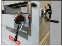
**TABLE & BED ROLL ADJUSTMENT** The idle bed rolls are conveniently adjusted from the front of the table. The eccentric cam allows you to raise and lower the bed rollers for optimum feeding results. A side handwheel adjusts the machine bed. The height is displayed by a ruler and indicator.
