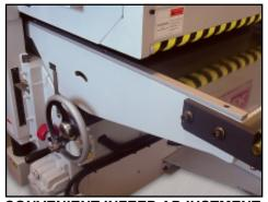
**CONVENIENT INFEED ADJUSTMENT** External handwheel directly next to the height scale provides quick and easy adjustment to the infeed bed.
