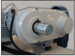
VARIABLE FEED SPEED Easy to access variable speed control allows you to dial in the correct feed rate for your surfacing application.
