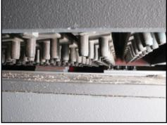
**SPRING LOADED CONVEYOR** Pressure spikes are in an overlapping layout to minimize gaps to ensure workpiece is held firmly.
