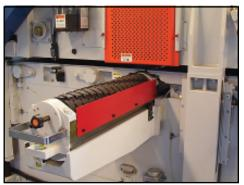
**FAST KNIFE CHANGE** Bottom head slides quickly out of the machine for fast knife change/rotation. Our 30mm wide knives provide a premium finish and require less time to change.
