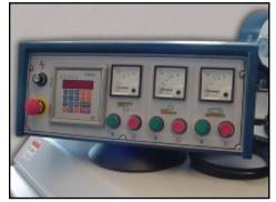
**SWIVEL CONTROL PANEL** East to access controls on swivel mount. Digital thickness control in Inch or MM (Inch to 3 decimal places for extra precision). Amp meters for each head and feed system.
