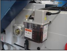
**AUTOMATIC LUBRICATOR** Auto oil lubricator provides metered and consistent lubrication to the Spring Feed System. Equipped with a manual lubricator to all elevation slideways.
