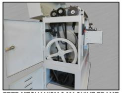
**FEED MECHANISM & MACHINE FRAME** Equipped with two feed speeds which are easily accessed through the side doors. A powerful chain feed system provide superior feeding results. The machine frame/table is mostly cast iron, with a heavy duty welded steel body.
