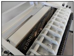
**SPIRAL INSERT KNIFE CUTTERHEAD** The spiral insert knife cutterhead provides a smooth finish with a quiet cutting operation. 4-sided solid carbide insert knives can be easily rotated for a new sharp cutting surface.
