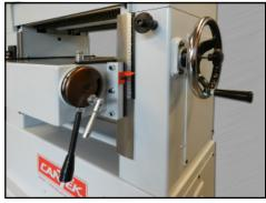
**TABLE & BED ROLL ADJUSTMENT** The idle bed rolls are conveniently adjusted from the front of the table. The eccentric cam allows you to raise and lower the bed rollers for optimum feeding results. A side handwheel adjusts the machine bed. The height is displayed by a ruler and indicator.
