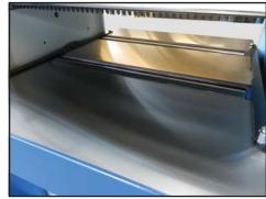
**IDLE BED ROLLS**Equipped with adjustable idle bed rollers which can be raised and lowered to facilitate in feeding difficult material. The rollers are directly opposed from the top driven feed rollers. The table surface is ground and polished to provide minimal friction.
