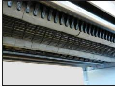
**SECTIONAL FEED & SAFETY SYSTEM** Equipped with sectional kickback fingers, sectional spring loaded serrated pressure rollers, and sectional pressure shoes for the most positive and safe feeding operations. Also equipped with double non-marking smooth outfeed top pressure rollers.
